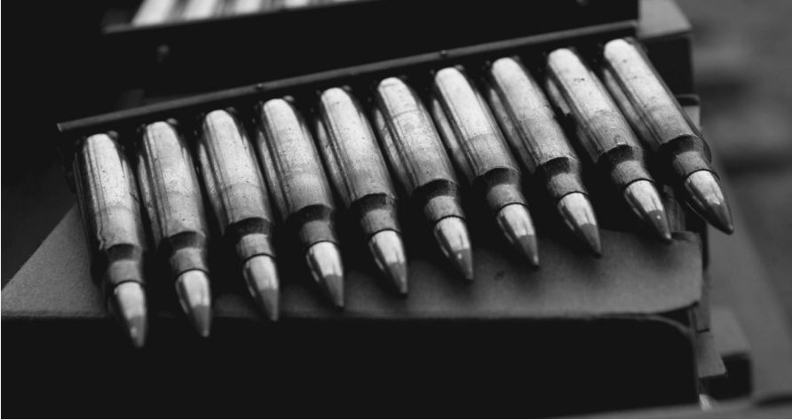
Figure 2.12 (See color insert.) Example of 5.56×45mm M855 “Green Tip” cartridges on stripper clips. Note the annealed casing neck. (U.S. Marine Corps image; photographer Cpl. Lydia M. Davey, USMC.)
